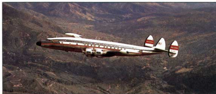
The final variant of the Super Constellation was the L-1049H, which featured a mixed passenger/cargo configuration with rapid role conversion as a prime feature.
